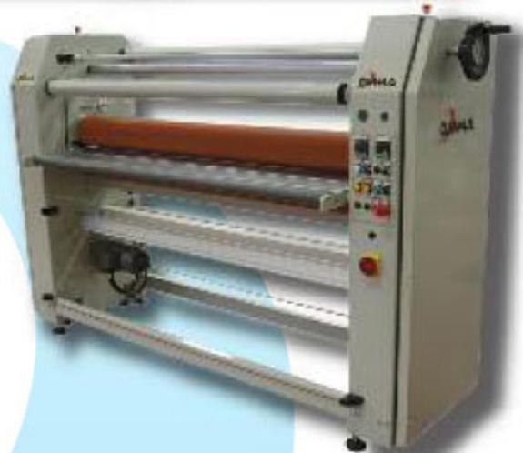
*It has a useful width of 1.600mm, simple but complete equipment, possibility to apply on top and bottom side at the same time and manual cut by the operator.*
